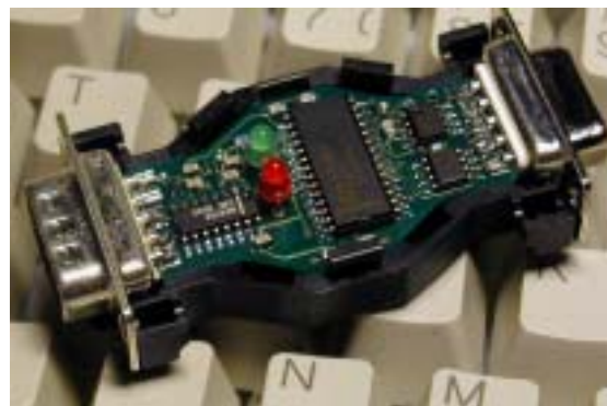
Top side (in enclosure) with Philips SJA1000.
